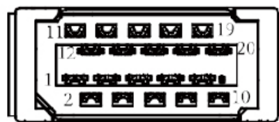
Real view of CN1 connecting terminals
